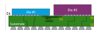
Conceptual drawings of fiber optic MCM using a high-density interposer for chip-to-chip interconnects. C4 die bumping pitch 55 \mu\text{m} and interposer BGA pitch 1.0mm.
