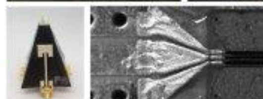
Conformal printing copper and silver for interconnects, 3D antennas, and wirebonds
